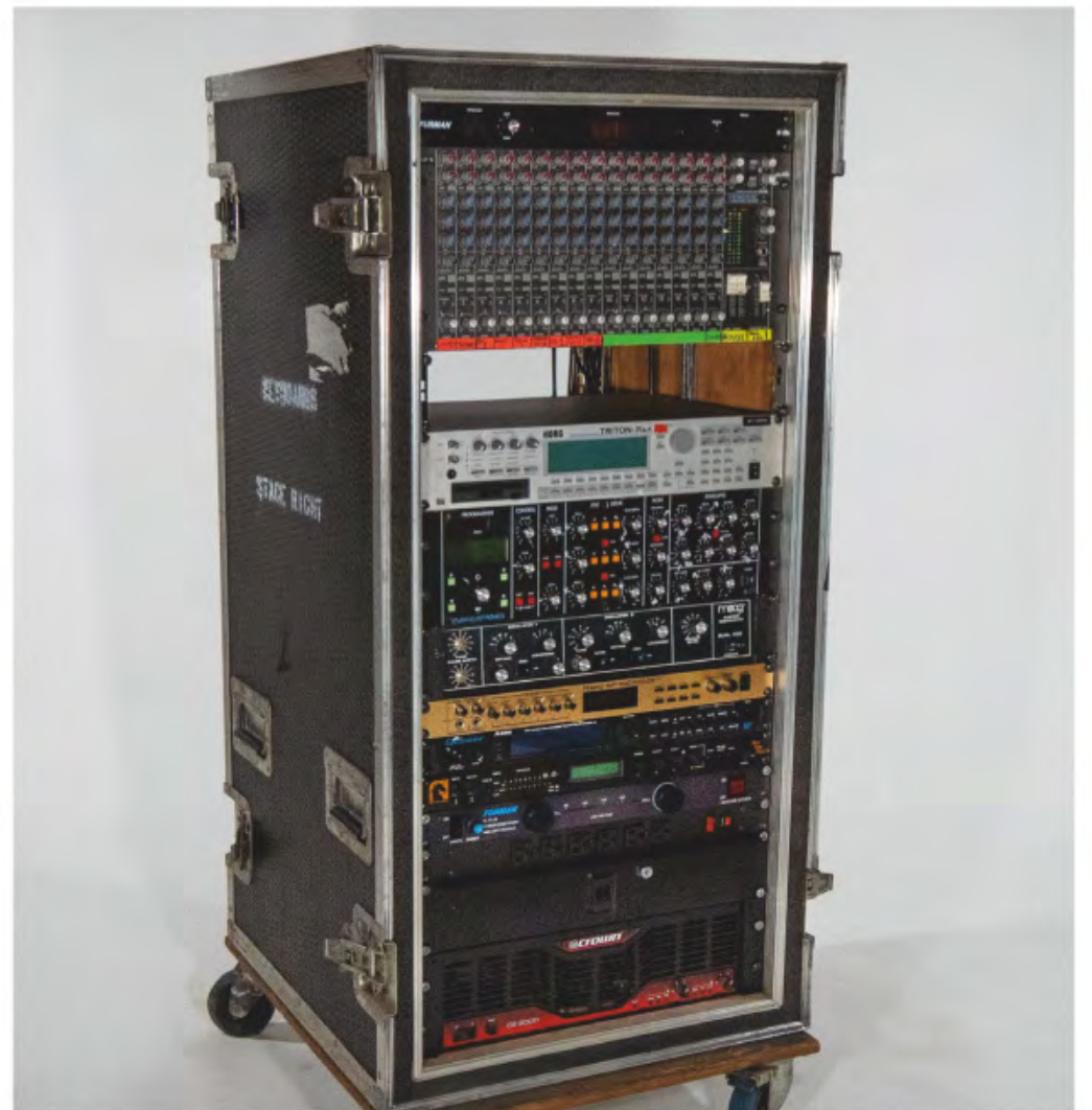
Fig. 4: Emerson's rack contained numerous synth modules and routed his mix to the front-of-house console
